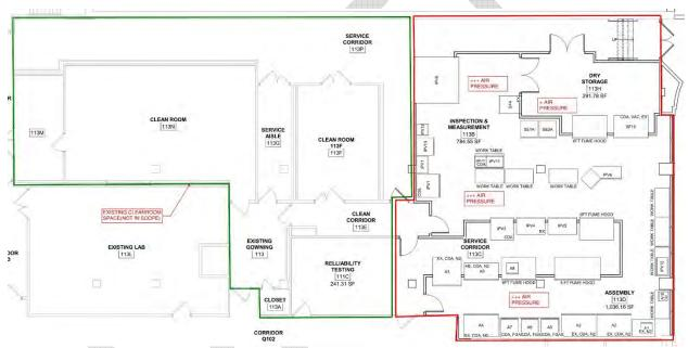
Figure 6: Cleanroom Pressurization Plan -Hybrid EEW
