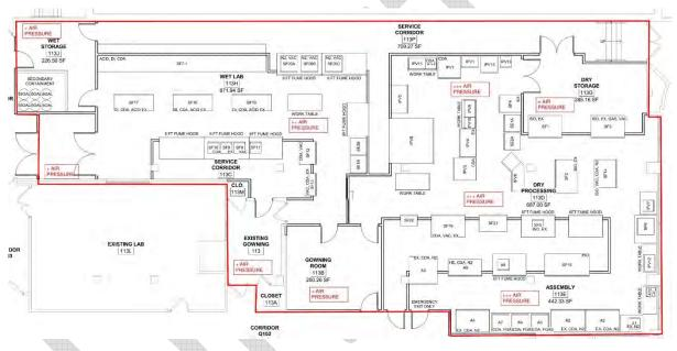
Figure 5: Cleanroom Pressurization Plan
