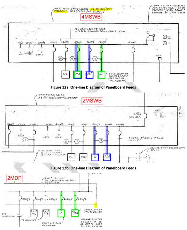
Figure 12c: One-line Diagram of Panelboard Feeds
