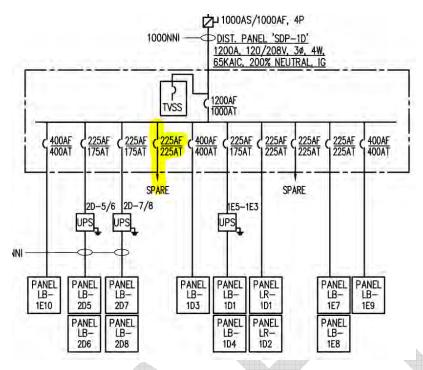
Figure 15: One-line Diagram of Power Distribution
