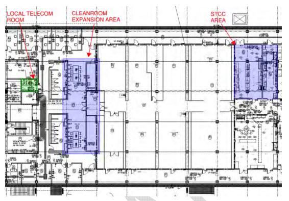
Figure 17: Telecommunications Room Location Plan
