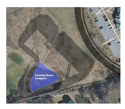
Figure 9. Schematic West Campus Basin Grading
