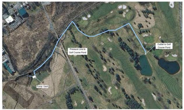
Figure 8. Reuse Water Pump System
