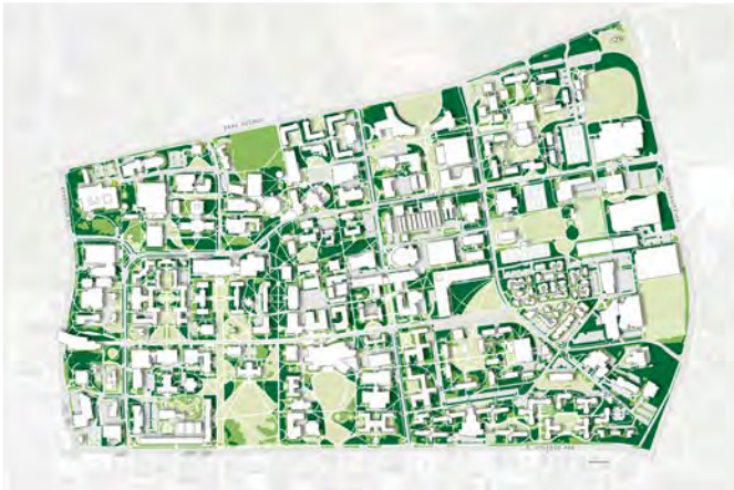
The dark green areas represent opportunities to maximize sustainable ground flora by transitioning underutilized landscape areas to higher performing landscape typologies.
